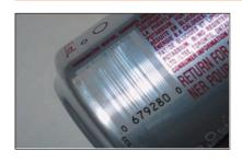
Using uncovered metal surfaces as a background or for the bars of a symbol. The specular reflectance of the substrate can cause problems, and a solid background must be printed to provide good contrast and eliminate this problem.
