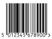
The width of the smallest bar or space is called the x-dimension; all other elements are multiples of this dimension.
