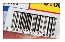
Missing bars or horizontal white lines crossing the bar code because of faulty print heads used for on demand printing.
